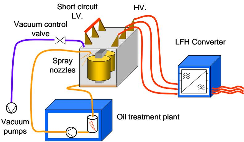
In order heat up both low and high voltage windings, a frequency of approx. 1 Hz is applied to the transformer. With the combination of LFH drying and the conventional hot oil spray method the whole transformer can be heated very uniform. The LFH system is heating the windings from the inside and the hot oil spray supports the heating process by heating outer parts of the insulation system.
