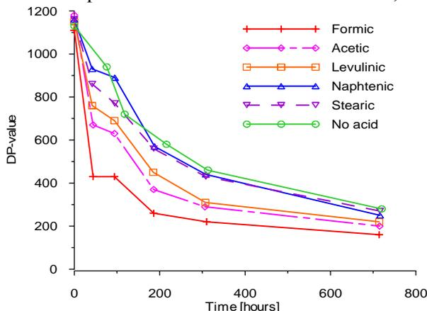
**Figure 2: Ageing of paper at 130°C in oils with an acidity of 0,4 with x % water in**
