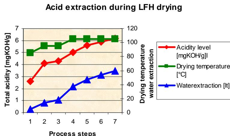
**Figure 5: Acid and moisture extraction during the LFH drying process**
