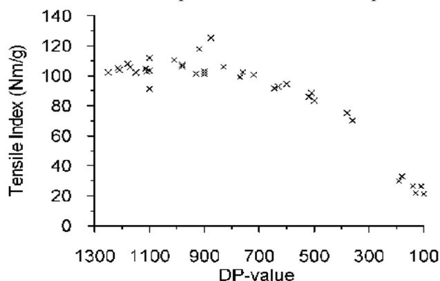
Paper (and pressboard) consists mainly of cellulose and some percent of hemicellulose and lignine. The reduction in mechanical strength is due to chain scissions of the cellulose molecules, on average having a chain length of 1000-1200 polysaccharide rings in series – denoted degree of polymerisation (DP) - when the paper in the transformer is new. The tensile strength depends on the DP as shown in figure 1. Conventionally a DP value of 200 is used as an end of life criterion
